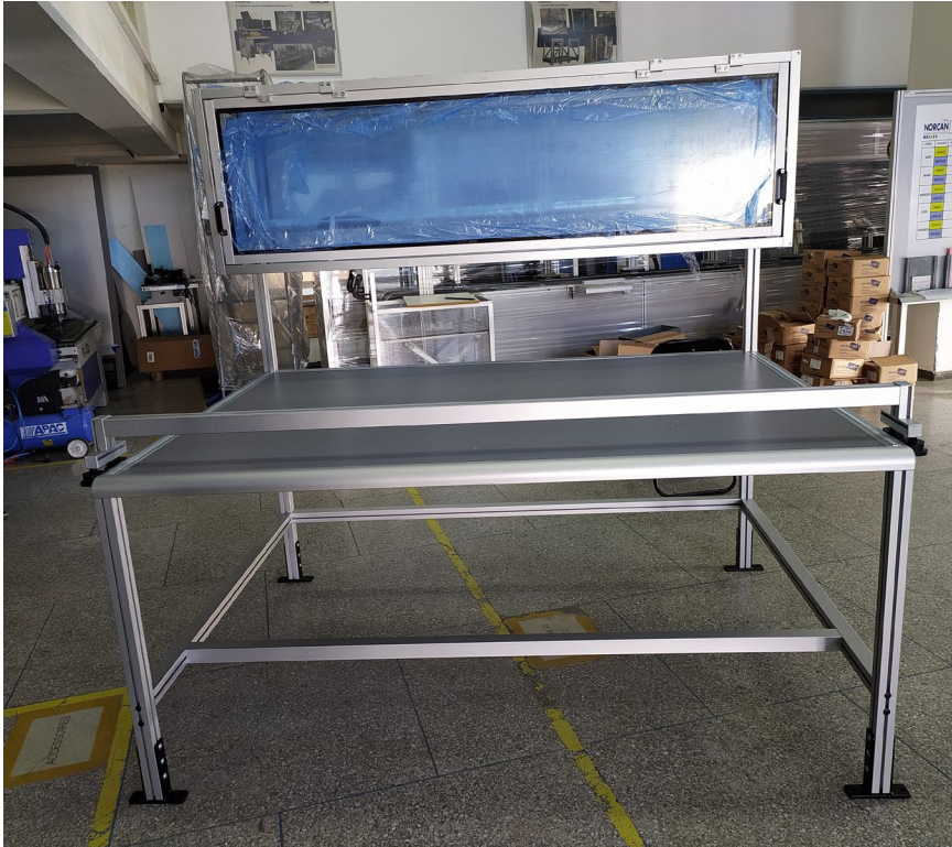
Norcan Morocco - Control station for hydraulic circuits of cars With an extension board for long sheaths
